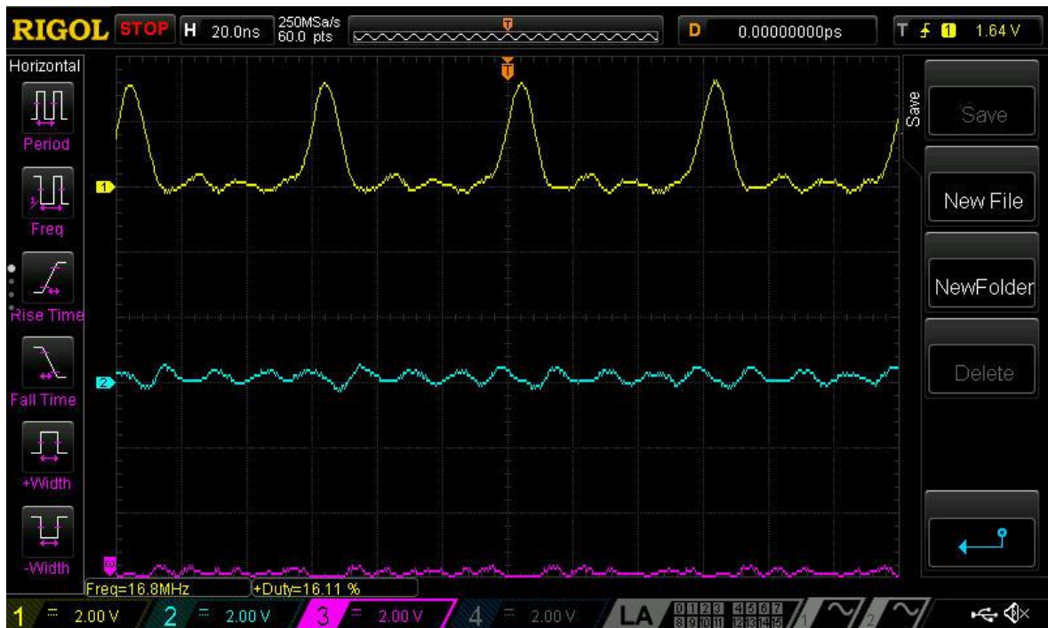
Figure 7. Output Waveforms at Period = 60 ns, Pulse Width = 10 ns, DC = 16.7 % (Correct Functionality)
