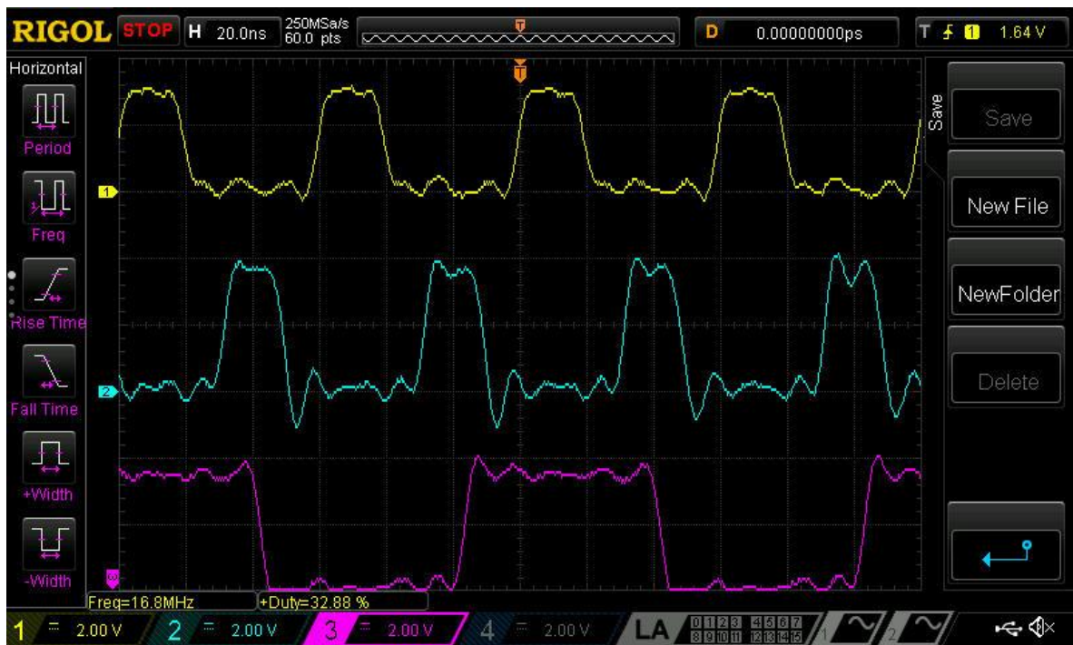
Figure 8. Output Waveforms at Period = 60 ns, Pulse Width = 20 ns, DC = 33.3 % (Incorrect Functionality)
