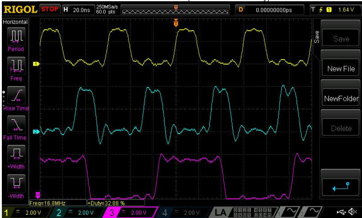
2. Period is 60ns. Pulse width is 20ns DC = 33.3% (Incorrect functionality)
