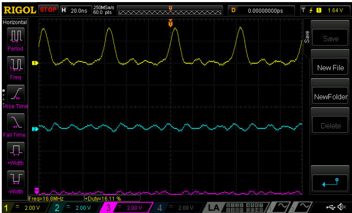
2. Period is 60ns. Pulse width is 20ns DC = 33.3% (Incorrect functionality)
