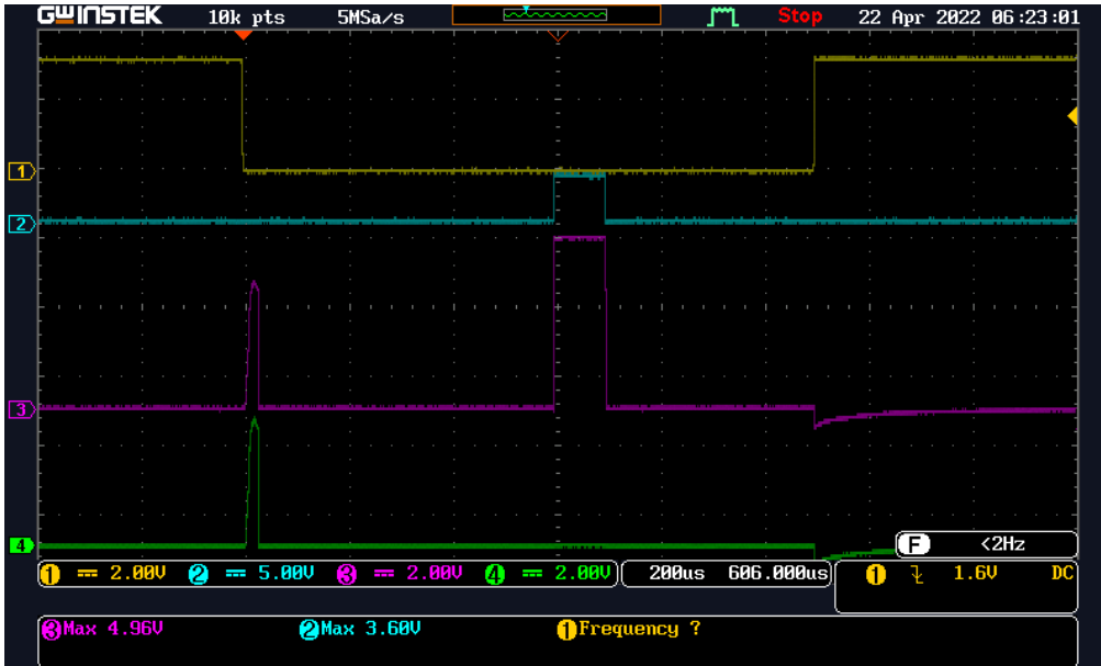
Figure 6 Glitch at HV_GPOx, decay = 1 (Slow decay)
