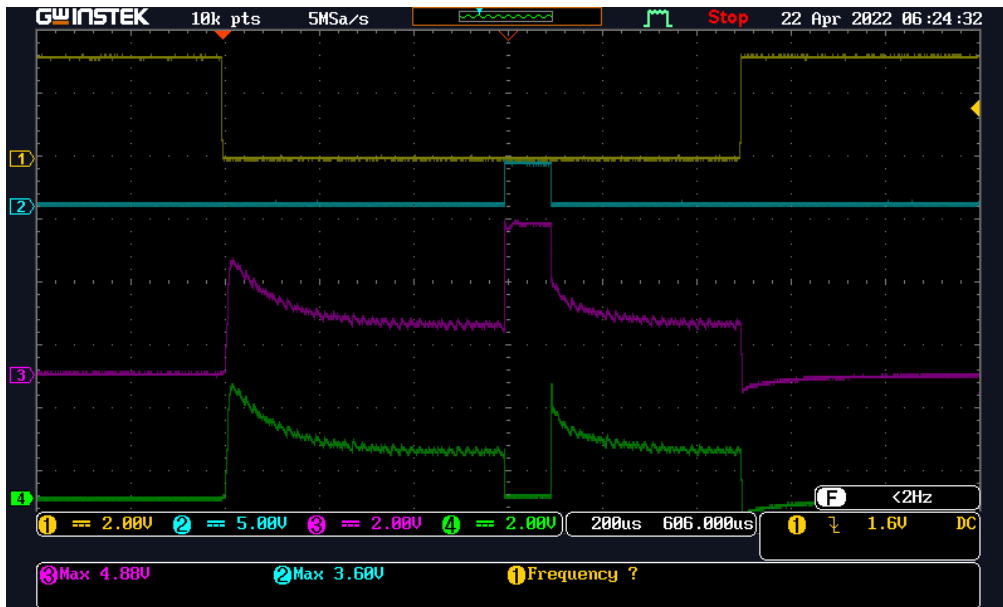
Figure 7 Glitch at HV_GPOx, decay = 0 (Fast decay)
