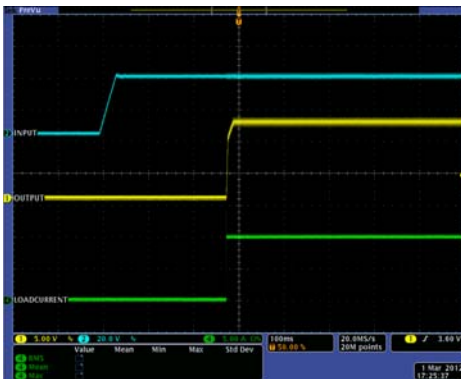
FIGURE 18. FULL LOAD START-UP, CH1: OUTPUT VOLTAGE, CH2: INPUT VOLTAGE, CH4: LOAD CURRENT
