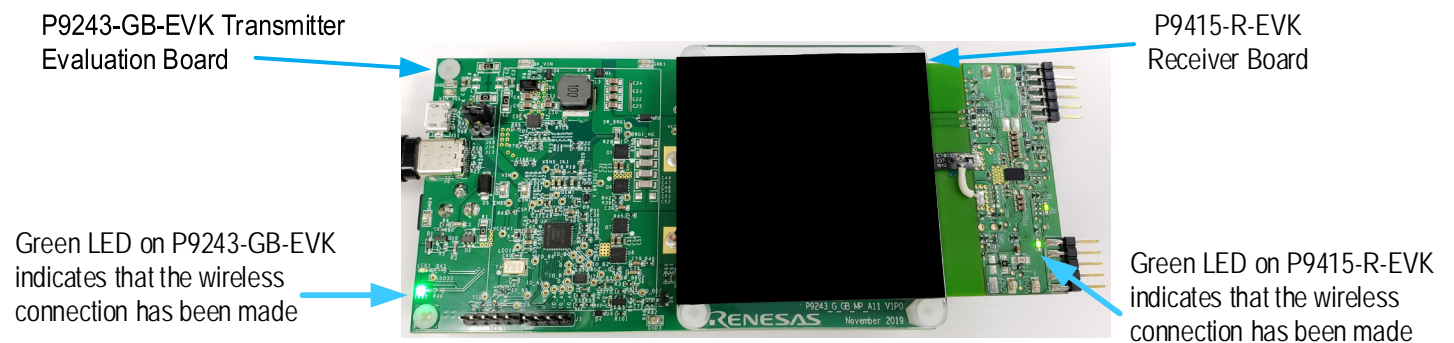
Figure 7. Evaluation Kit Connections using the P9415-R-EVK Receiver Evaluation Board
