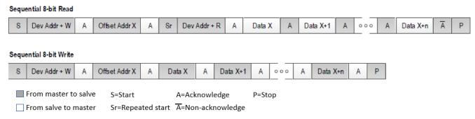
Figure 1. I2C 1-Byte Offset Mode Slave Sequencing
