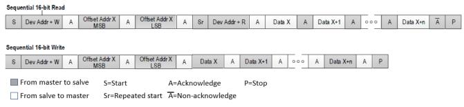
Figure 2. I2C 2-Byte Offset Mode Slave Sequencing
