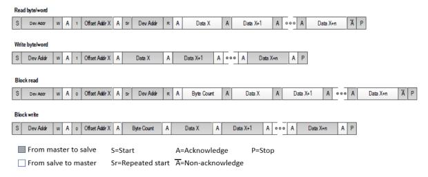
Figure 4. I2C Slave Timing Diagram
