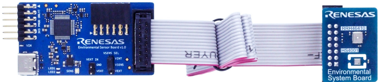
Figure 3. Using a 14-Pin Ribbon Cable to Increase Distance between Communication and Sensor Board
