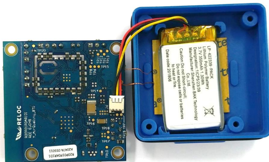
Figure 3: Coil and battery positioning.
