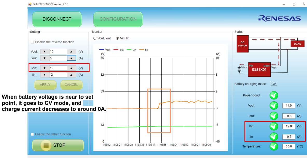
Figure 13. Fully Charging Information in GUI
