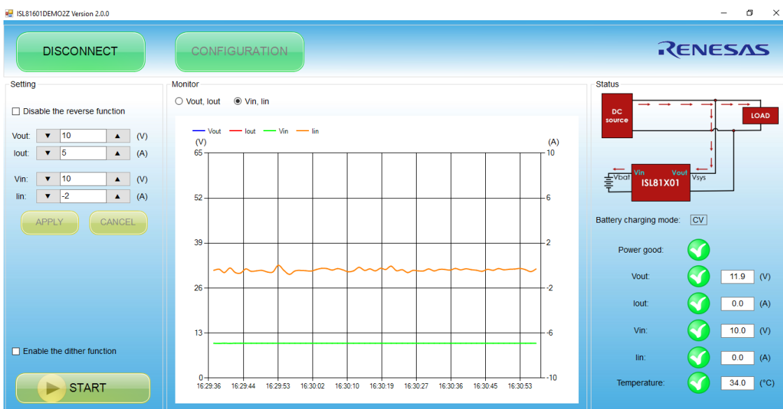
Figure 7. Precharge Complete Information in GUI
