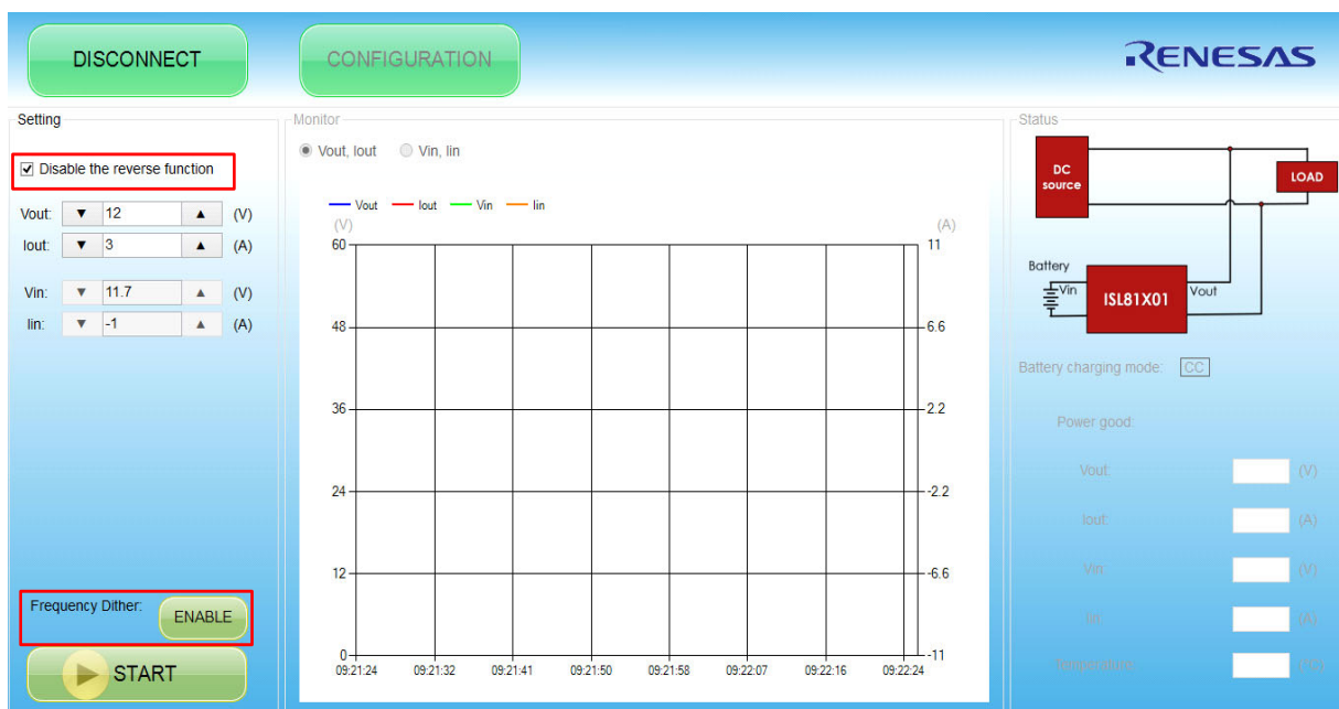
Figure 17. Disable Reverse Operation and Enable Dither Functions
