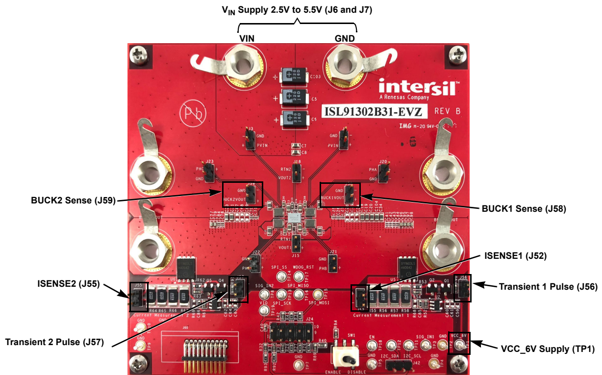
Figure 12. ISL91302B31-EVZ Load Transient Measurement Connections (Top View)
