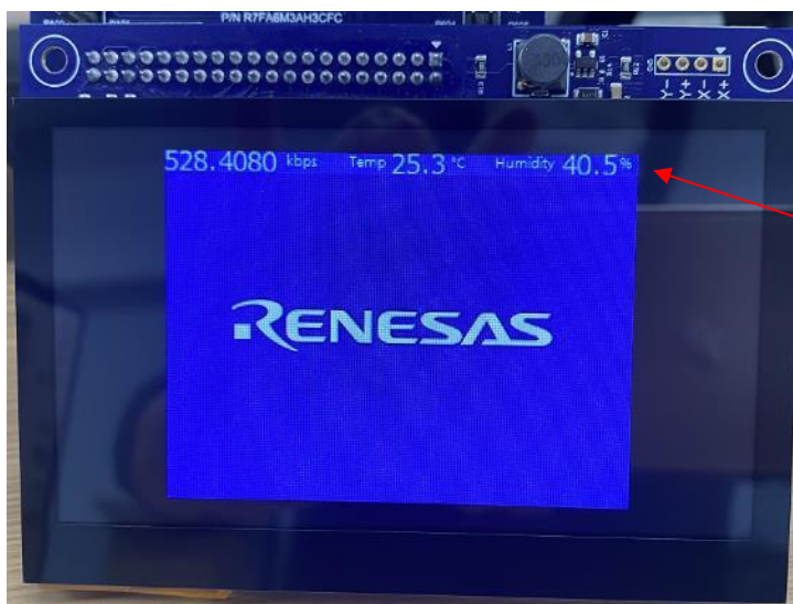
Display of throughput, temperature and humidity
