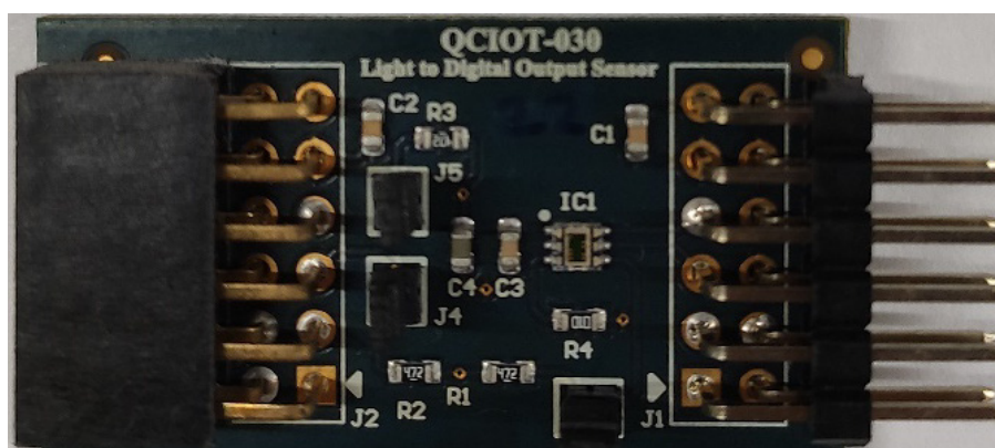
Figure 1. QCIOT30-ISL76683EVZ PMOD Board (QCIOT-030)
