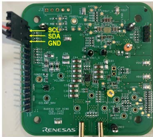
Figure 23. USB-I2C Bridge Connected to I2C Terminal J1 of RA9530-R EVK Board
