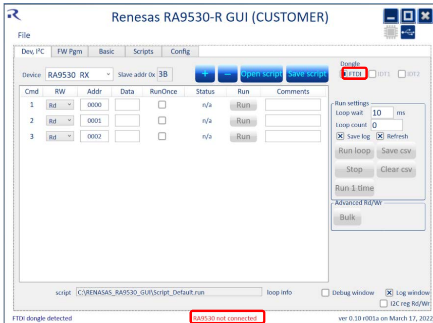
Figure 25. USB-bridge is Detected; RA9530 is Not Connected
