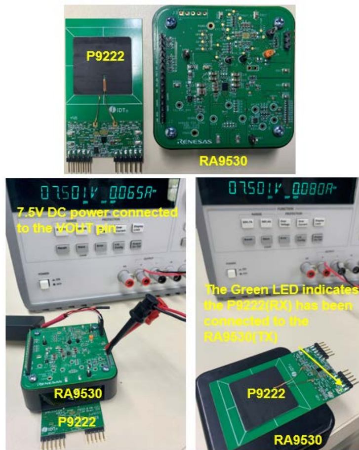
Figure 16. Evaluation Kit Connections for TRx Mode Test
