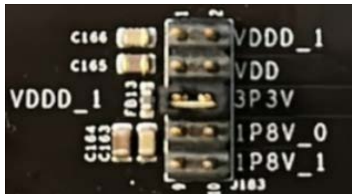
Figure 6. Power Source Selector for V_{DDD_1}
