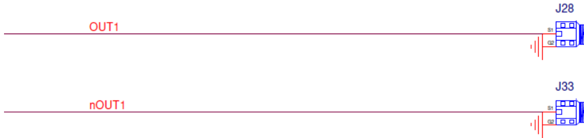
Figure 15. Output Clock DC-Coupling
