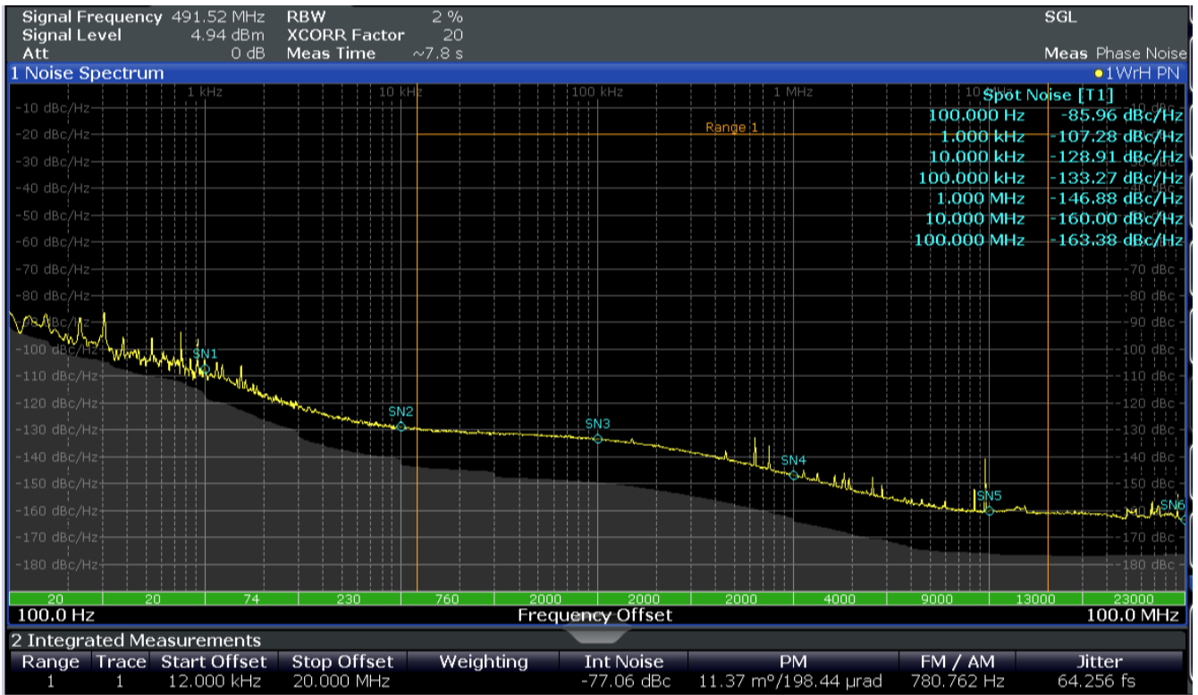
Figure 32. Phase Noise 491.52MHz Output Synthesizer Mode
