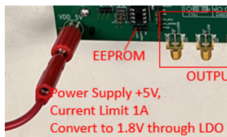
Figure 4. External 5V Board Input
