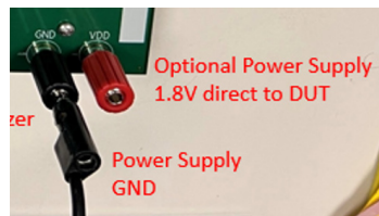
Figure 6. J90 Board Input
