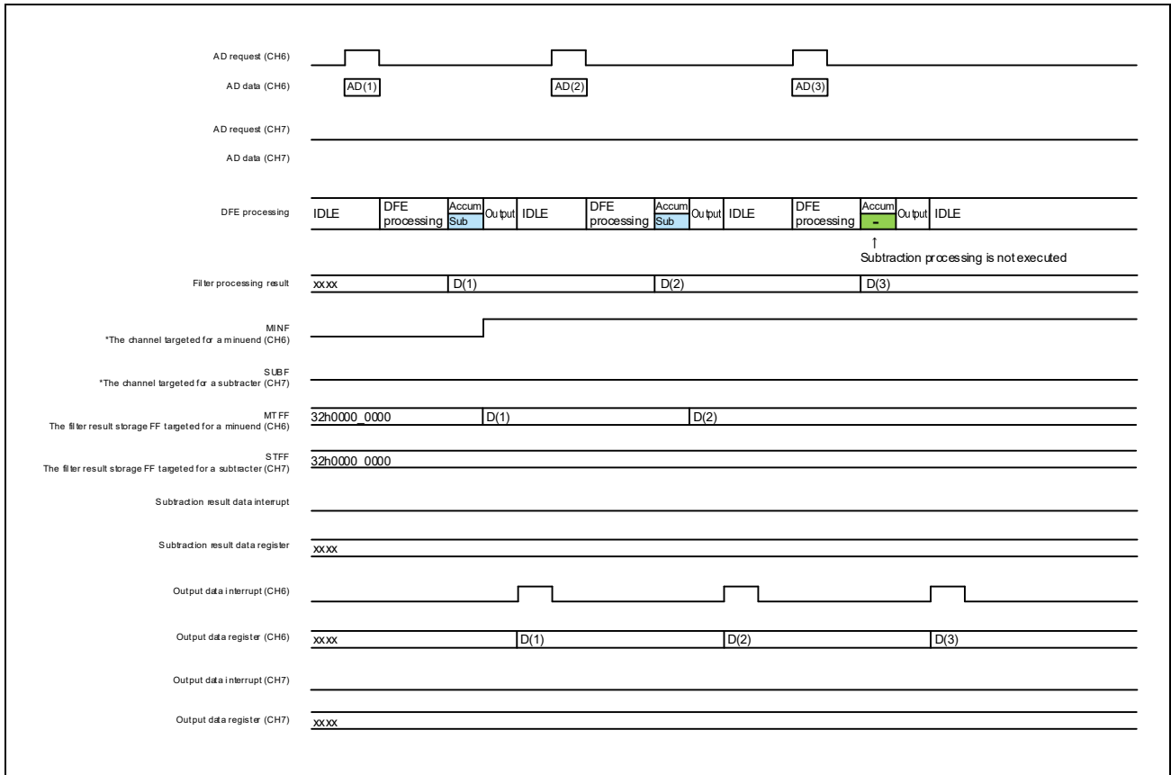
Figure 37.68 Subtraction Processing (when Processing for Only a Subtrahend Channel is Executed and Finished)
