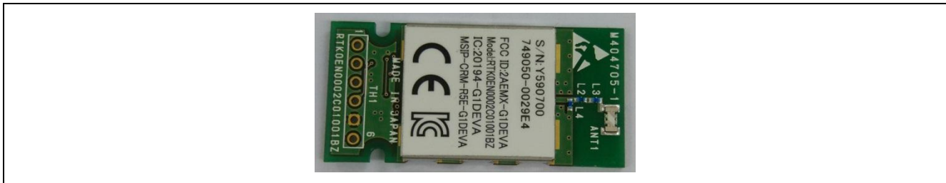
Figure 2.4 Circuit Board of RL78/G1D Module
