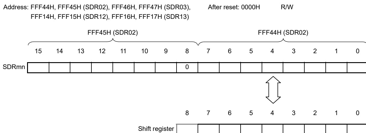
Figure 17 - 4 Format of Serial data register mn (SDRmn) (mn = 02, 03, 12, 13)
