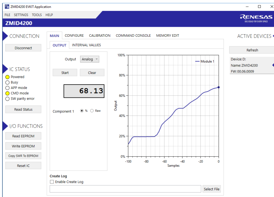
Figure 11. “OUTPUT” Tab – Analog Output Example
