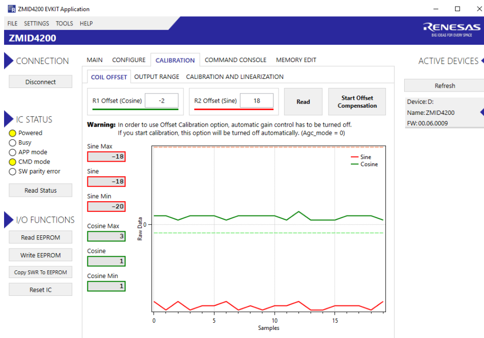
Figure 22. “COIL OFFSET” Tab – ZMID4200 Example
