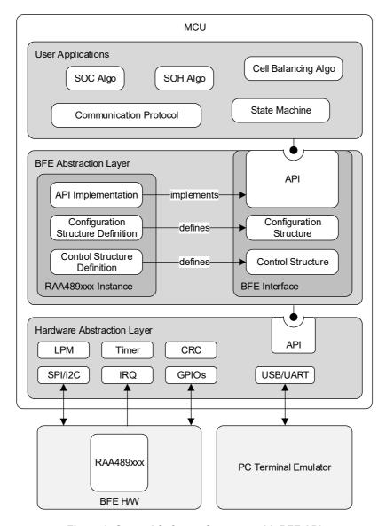
Figure 2. General Software Structure with BFE API
