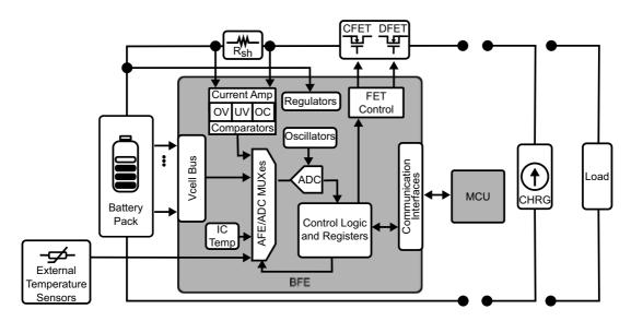
Figure 1. General Block Diagram of Battery Management System
