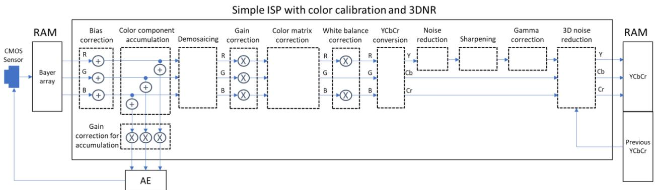
Figure 1-1 Block diagram of Simple ISP with color calibration and 3DNR
