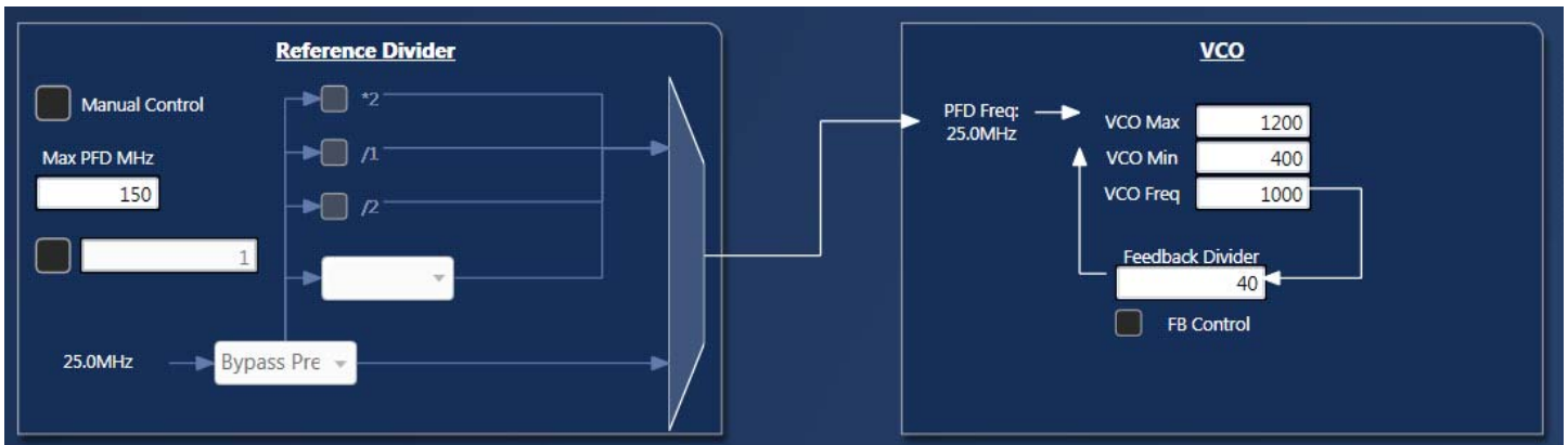
Figure 16. Phase Locked Loop (PLL3)
