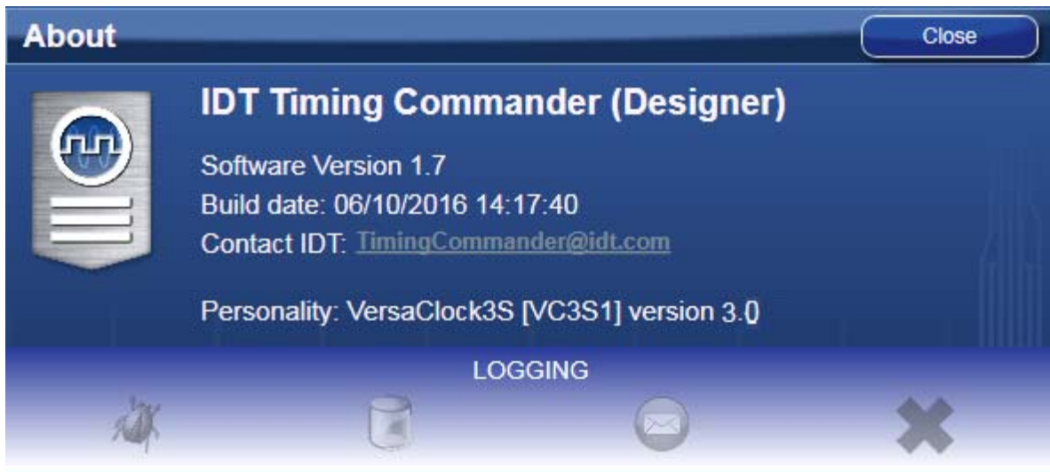
Figure 46. From About icon, an E-mail can be Generated to IDT with Option of Attaching a Log File
