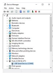
Figure 2. The ZMID-COMBOARD Appears as a Serial Device
