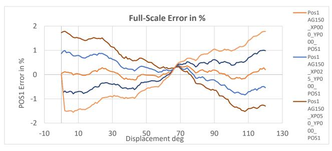
Figure 6. Accuracy with Linearization at 1.5mm Airgap and Effects of Displacement in X
