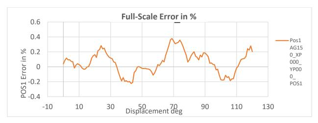
Figure 4. Accuracy with Linearization at 1.5mm Airgap (AG150)
