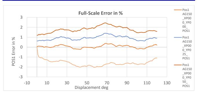
Figure 7. Accuracy with Linearization at 1.5mm Airgap and Effects of Displacement in Y
