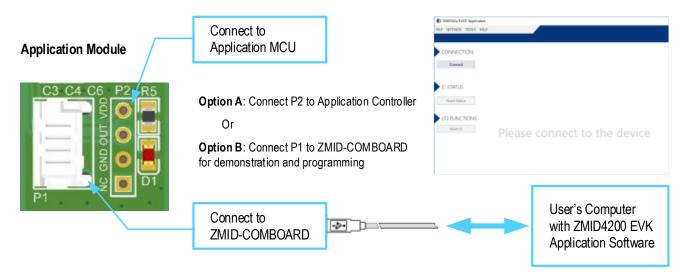
**Figure 1. Application Module Connections**
