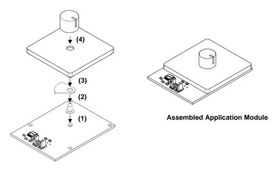
Figure 2. Target Holder Assembly
