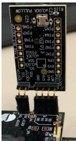
Figure 11. Connection between Socket Board and Evaluation Board
