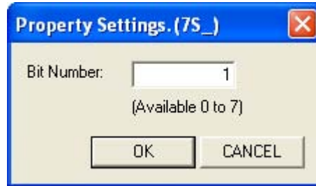
Figure 6-33. Property Settings Dialog Box (for the [7-Segment LED Jumper (Bit Type)] Panel)
