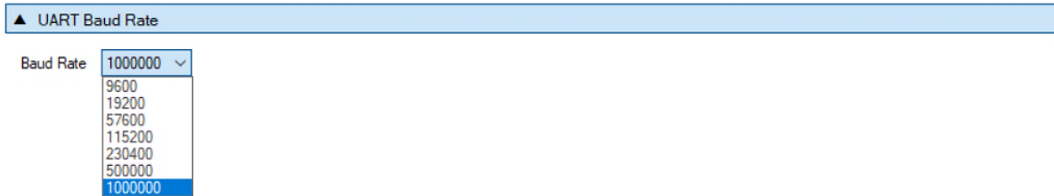
Figure 80: UART Baud Rate - DA1469x
