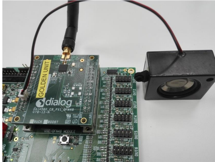
Figure 169: Speaker Connection for Audio Test.
