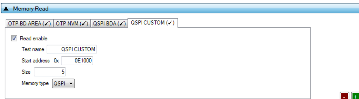
Figure 103: Memory Read Test - DA1469x
