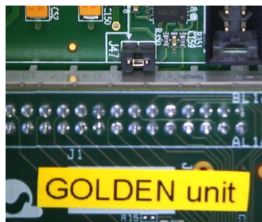
Figure 129: Jumper J47 Added Next to Golden Unit Socket
