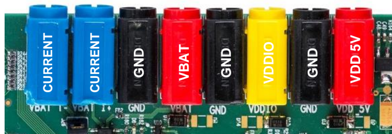
Figure 4: PLT Hardware Power Connections
