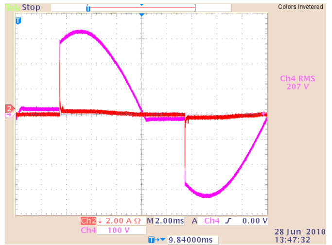
FIGURE 19B. IGNITION ANGLE IS 60°
