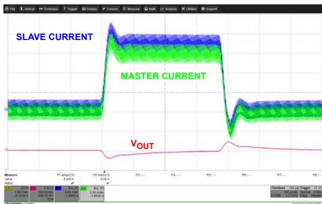
FIGURE 5. DUAL ISL70002SEH SHARING of 0 TO 14A LOAD CURRENT TRANSIENT STEP, V_{IN} = 3.3V , V_{OUT} = 1.0V , 1MHz
