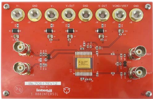
FIGURE 12. ISL70517SEHEV1Z EVALUATION BOARD
