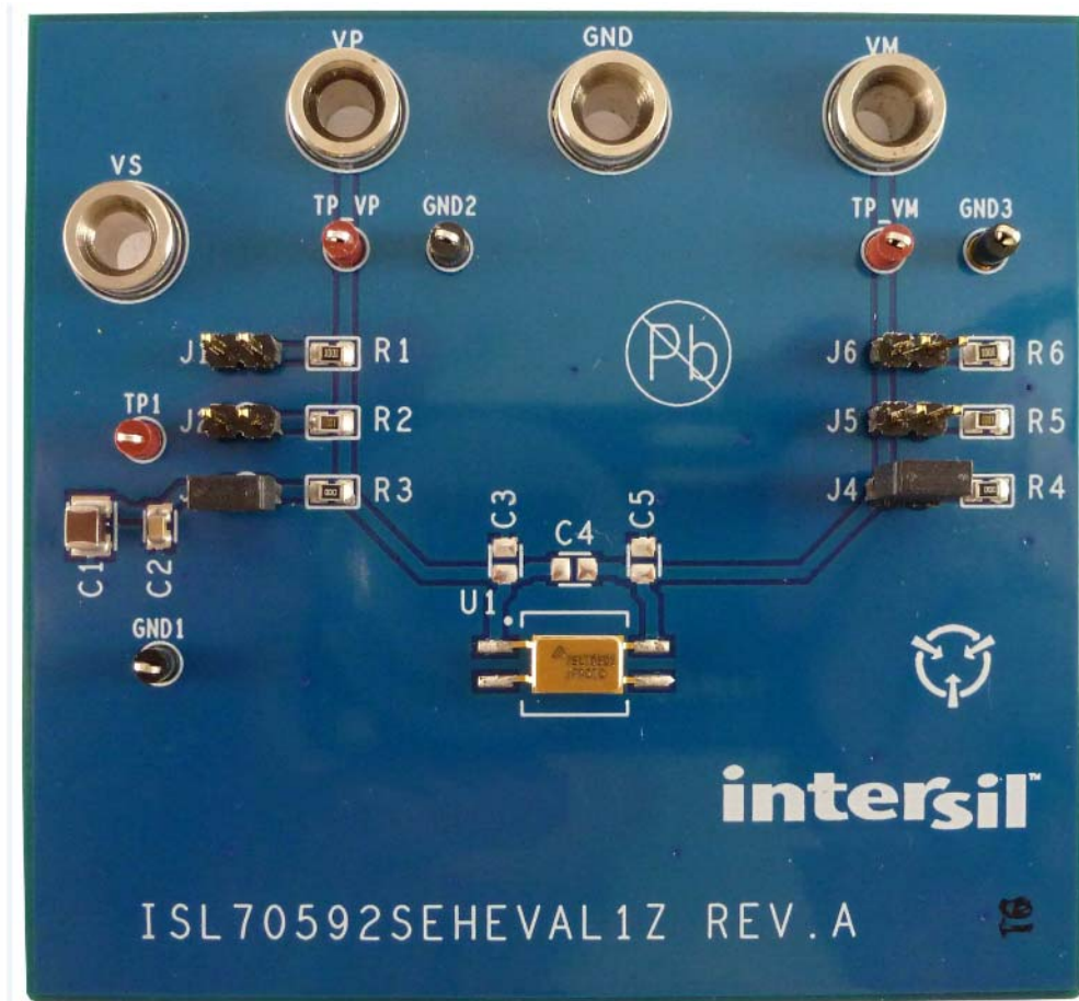
Figure 3. ISL70592SEHEVAL1Z Evaluation Board
