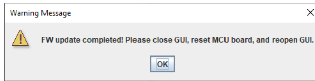
Figure 28. iRADNavigator MCU Firmware Online Update - Program Firmware
