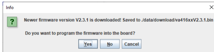
Figure 27. iRADNavigator MCU Firmware Online Update - Program Firmware
