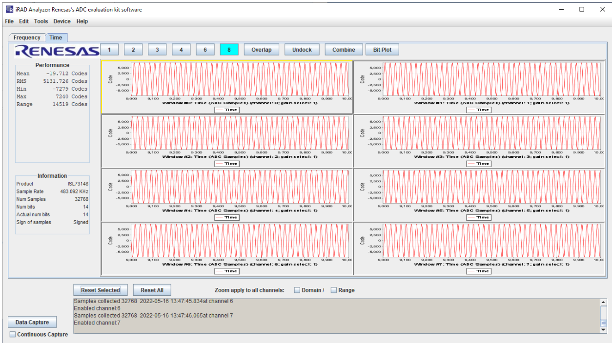
Figure 17. iRADAnalyzer 8-Channel Time Domain Plot
