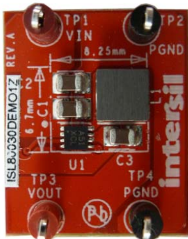
FIGURE 2. ISL80030DEMO1Z TOP SIDE
