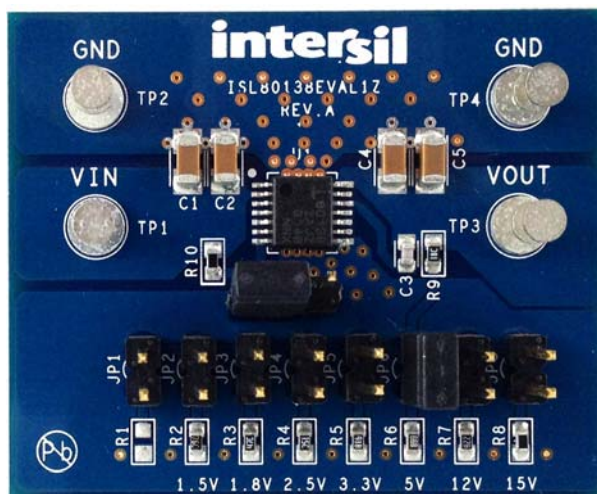
FIGURE 1. ISL80138EVAL1Z EVALUATION BOARD
