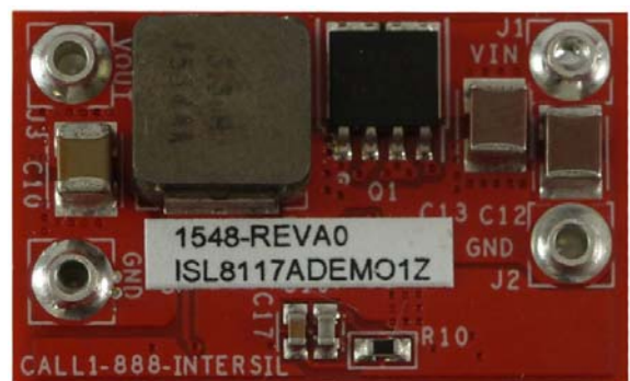
FIGURE 5. ISL8117ADEMO1Z BOTTOM SIDE
