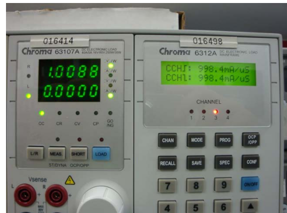
FIGURE 1. TYPICAL ELECTRONIC LOAD SETUP
