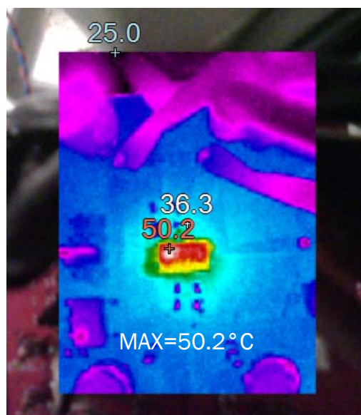
FIGURE 21. THERMAL IMAGE AT V_{IN} = 5V , V_{OUT} = 1.2V , I_{OUT} = 5A , f_{SW} = 1.6MHz , T_A = +25^\circ C , FREE AIR 0 LFM
