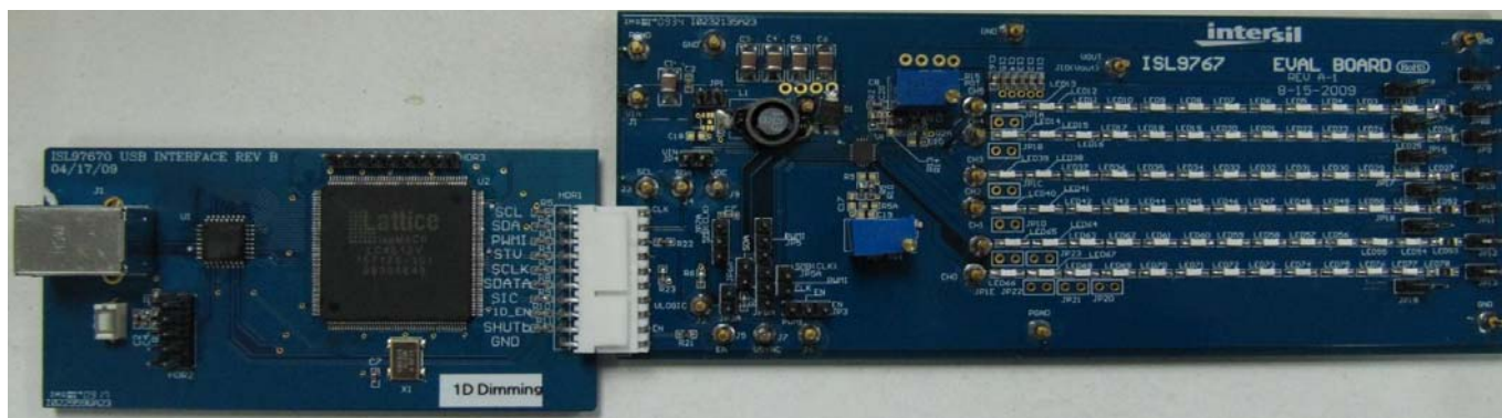
FIGURE 4. I 2 C INTERFACE BOARD CONNECTED TO ISL97674IRZ-EVAL EVALUATION BOARD
