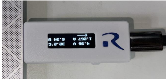
Figure 9. Flipping the Screen by Pressing the Button
