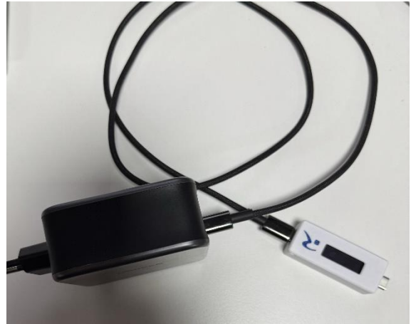
Figure 4. Receptacle Connection to Host Device
