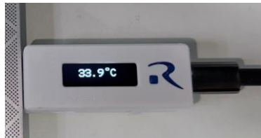
Temperature Screen (Four Presses)
