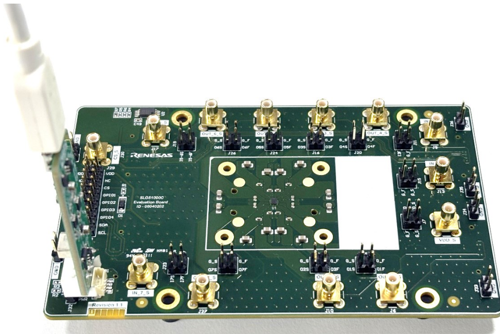
Figure 6. Evaluation Board with GreenPAK Serial Debugger
