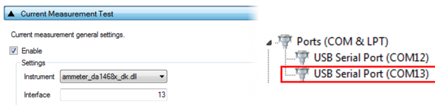
Figure 178: DA1468x DK PRO Current Measurement Settings
