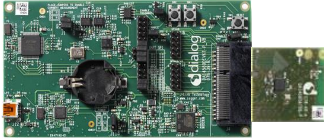
Figure 22: ProDK with a QFN40 DA14585
