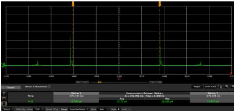
Figure 28: DA14585 Voice RCU Reference Design – Average Sleep Current
