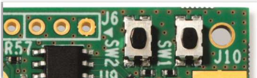
Figure 15: General purpose push buttons SW1, SW2 (populated at TOP)
