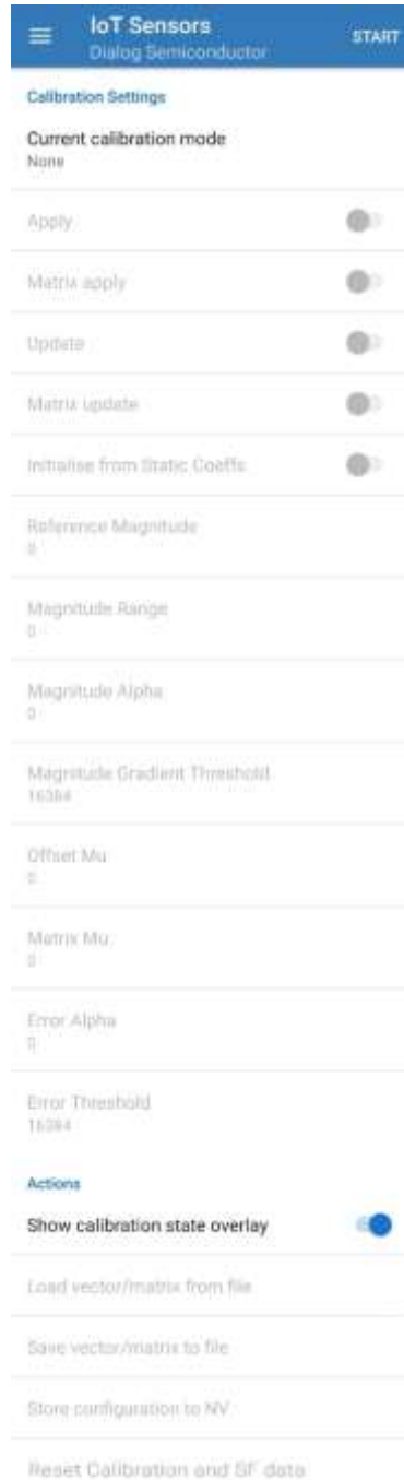
Figure 11: Calibration Settings of Dialog IoT Sensors App
